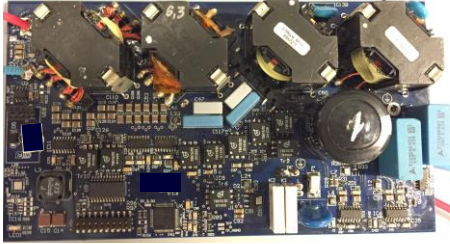
Fig. 2. Photo of the built PV microinverter prototype.
