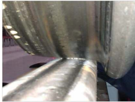
Fig. 29 Hollow wear on wheels of EMUs running in south China at a maximum of 350 km/h in 2011–2012 [42]. Laterally, x = 0.0 coincides with the NRC (also for similar figures later). (a) Profile development of a wheel and (b) light appearing in the contact gap between another hollow wheel and a rail.
