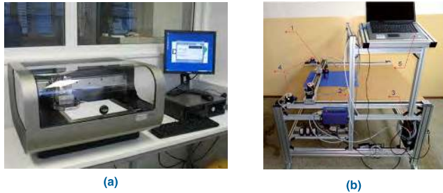
FIGURE 10. (a) Commercial DMP 2831 ink jet printer, (b) Setup of Inkjet printing with simultaneous sintering process on the textile substrate [63].
