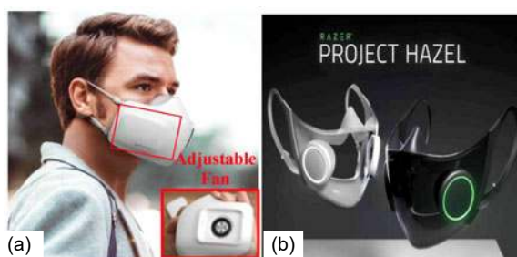
Fig. 10 PuriCare wearable air smart mask developed by LG Group (LG Group, 2020) (a) and a smart mask manufactured by Razer and equipped with an automatic ventilation system (Razer, 2020) (b)
