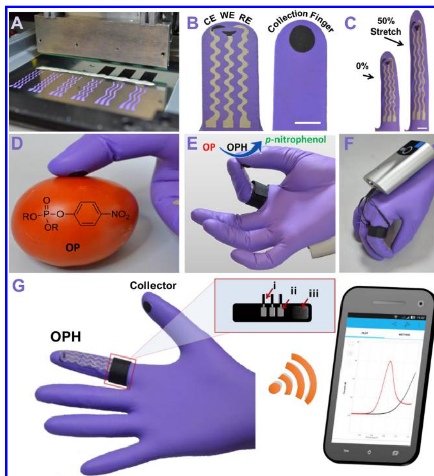
Figure 1. Flexible glove biosensor: fabrication, design and performance. (A) Image of the serpentine stencil design employed for printing the glove-based stretchable device. (B) Schematic of (left) the biosensing scan finger (index finger) containing smiling face shape carbon-based counter (CE), working (WE) electrodes and Ag/AgCl-based reference electrode (RE), and (right) collecting thumb finger with its printed carbon pad; scale bar 10 mm. (C) Photographs of the biosensing index finger under 0% (left) and 50% (right) linear stretch; scale bar, 10 mm. (D) On-glove swiping protocol for sampling chemical threat residues from tomato and stainless steel surfaces. (E) On-glove sensing procedure by joining the index (scan) and thumb (collector) fingers to complete the electrochemical cell. (F, G) Photographs of the wearable glove biosensor, consisting of a sensing finger, containing the immobilized OPH enzyme layer, and the collector/sampling finger. The electrodes are connected via an adjustable ring bandage to the portable potentiostat (attached to the back of hand) for on-site detection with wireless communication to a smartphone for rapid presentation of the voltammetric results. (Inset) Schematic of the interface between potentiostat and glove sensor. The connections consist of a (iii) velcro fabric containing (ii) the aluminum-tape based pins that are adjusted as a ring with the glove sensing connectors and (i) the wiring with the potentiostat.
