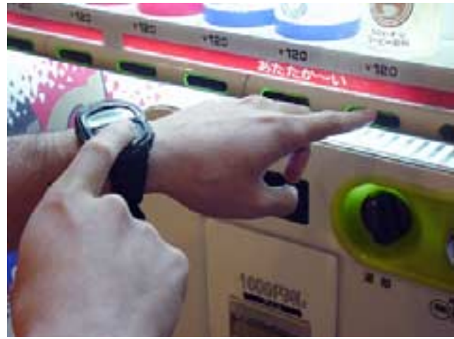
Figure 11: Wearable Key with Fingerprint Reader (ENVISIONMENT): The owner of the key is identified by the fingerprint reader, and the encrypted biometrics features are sent to the keyhole.
