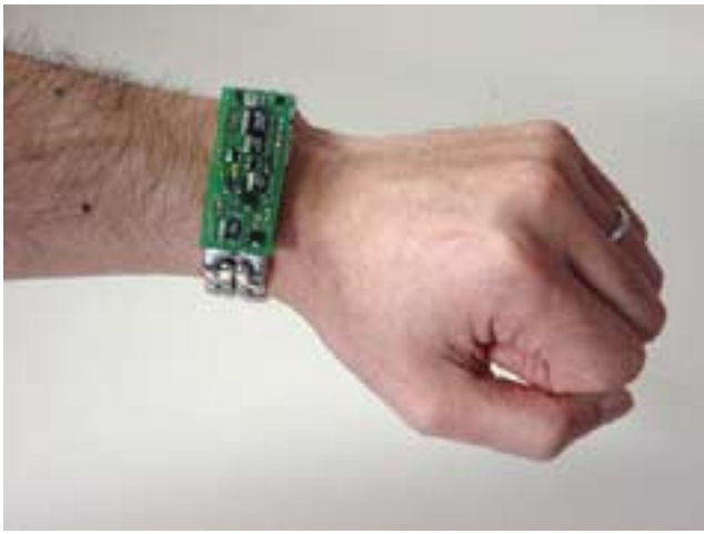
Figure 8: Wearable Key: The TouchNet module is put into a wristwatch-like unit. The user wears the key with the electrode of the TouchNet module in contact with the body.
