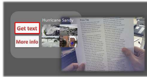
Fig. 5. A sample view of visual feedback. The red bounding rectangle indicates the user is currently selecting the "Get text" button.
