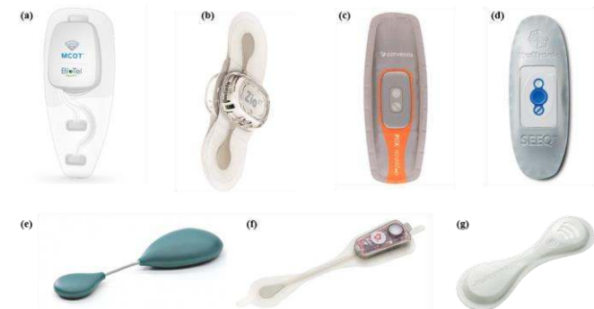
Fig. 6. Commercial ECG patches used in clinical trials and in COVID-19, (a) MCOT (BioTelemetry, Pennsylvania, USA), (b) Zio XT (iRhythm, California, USA), (c) NUVANT (Corventis, California, USA), (d) SEEQ TM MCT patch (Medtronic, Dublin, Ireland), (e) Savvy (Ljubljana, Slovenia), (f) CAM TM (Bard/Dx, Washington, USA), (g) VitalPatch (VitalConnect, California, USA).
