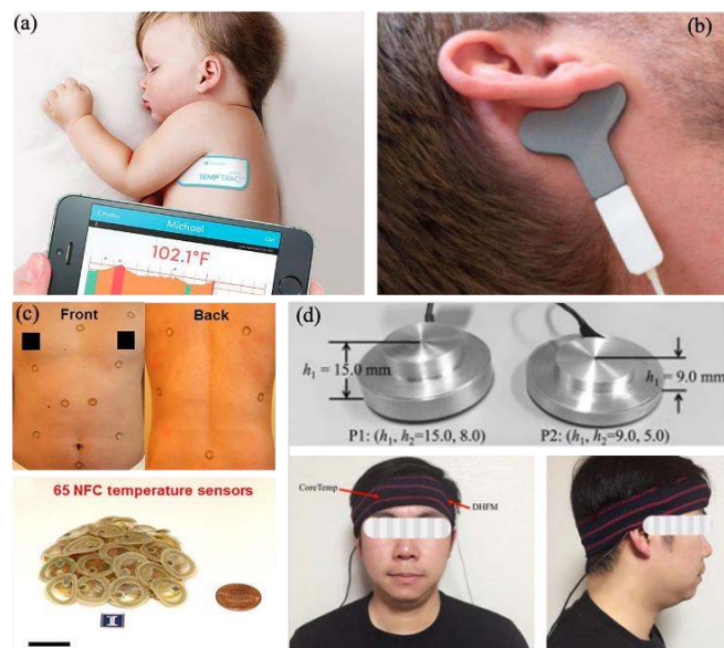
Fig. 9. Wearable temperature monitoring: (a) TempTraq® temperature Bluetooth-enabled patch [145], (b) foam-based flexible thermal sensor [144], (c) epidermal wireless thermal sensor array [142], and (d) headband thermometry [143].
