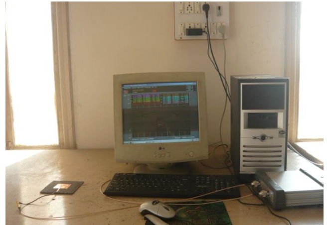
Figure 6 Measurement set-up of return loss
