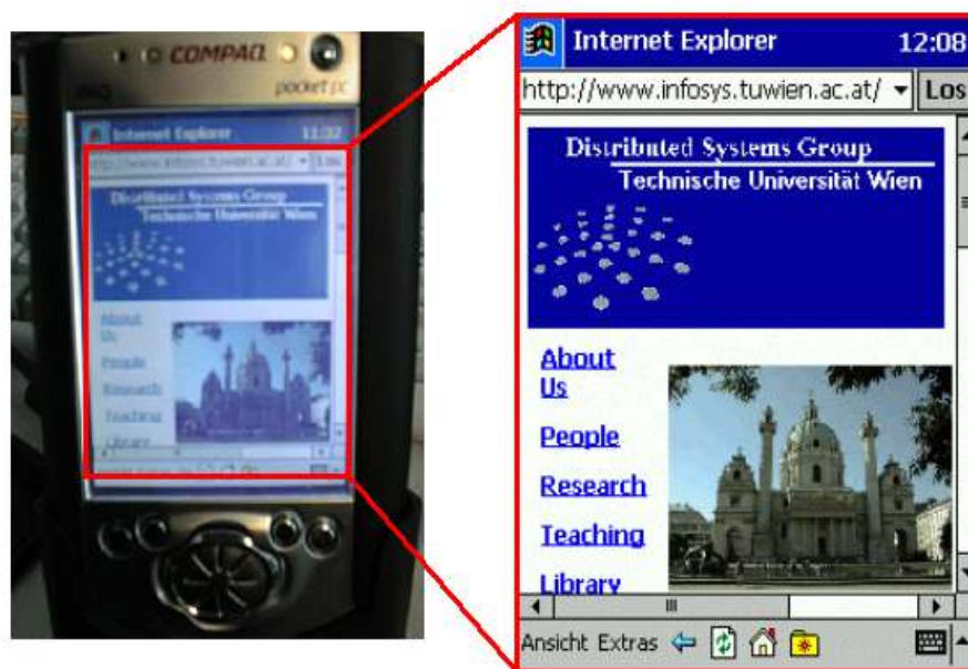
Figure 2.2: The difficulty of supporting small displays: The DSG homepage as seen on an iPAQ PDA
