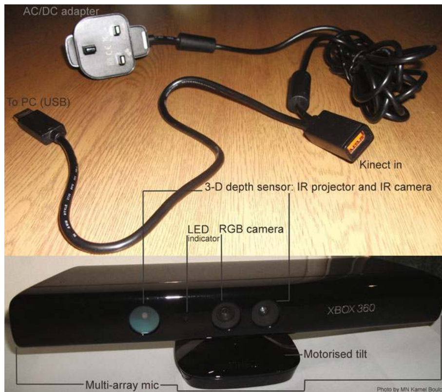
Figure 1 Anatomy of Microsoft Kinect.
