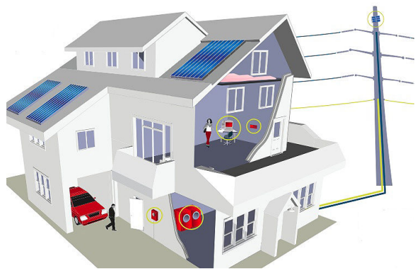
Fig. 1. Internet of Things in domestic environments: appliances and utilities can be monitored and controlled in near-realtime using smart embedded systems with IP connectivity.
