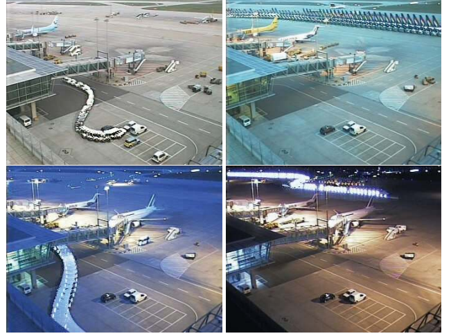
Figure 3. Four extracted tubes shown “flattened” over the corresponding backgrounds from Fig. 2. The left tubes correspond to ground vehicles, while the right tubes correspond to airplanes on the runway at the back. This figure is best viewed in color.
