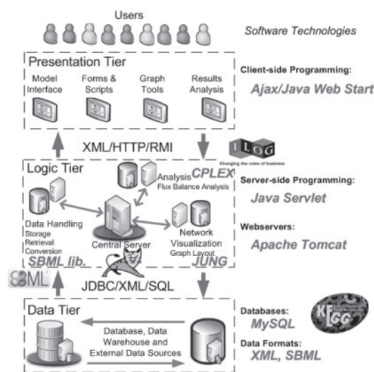
Fig. 1. Three-tier architecture of the WEbcoli system. Several software technologies and libraries are used to implement the configured layers including data, logic and presentation.
