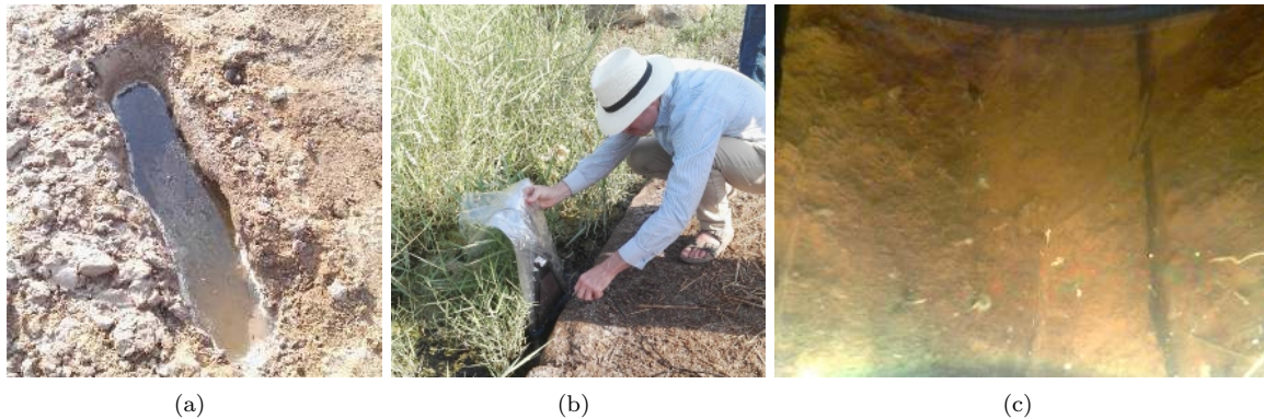
Fig. 10. (a) An overflooded trench where the wedge can be used; (b) a wedge being used for observing the side of a flooded area; (c) image acquired underwater.
