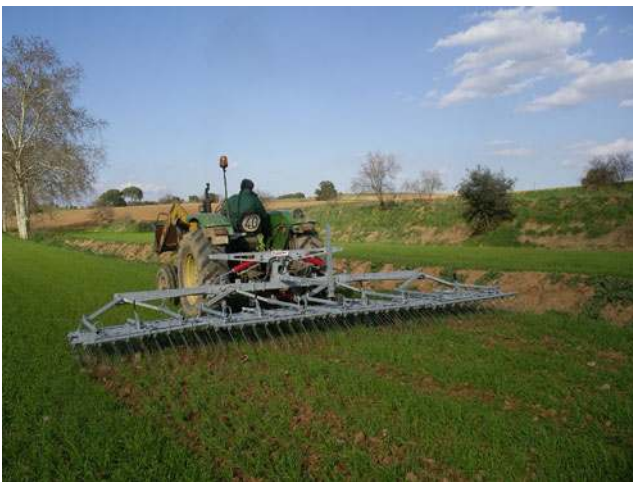
Fig. 1 Organic farmer using a weed harrow. Most organic farmers use weed harrows as a direct physical method to control weeds. Weed harrows till the soil surface, uprooting and/or covering the weed seedlings with soil
