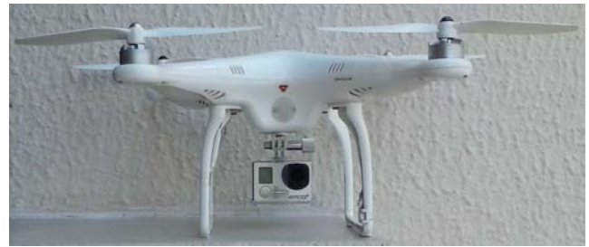
Figure 2. DJI Phantom with a GoPro Hero3 Silver Edition.
