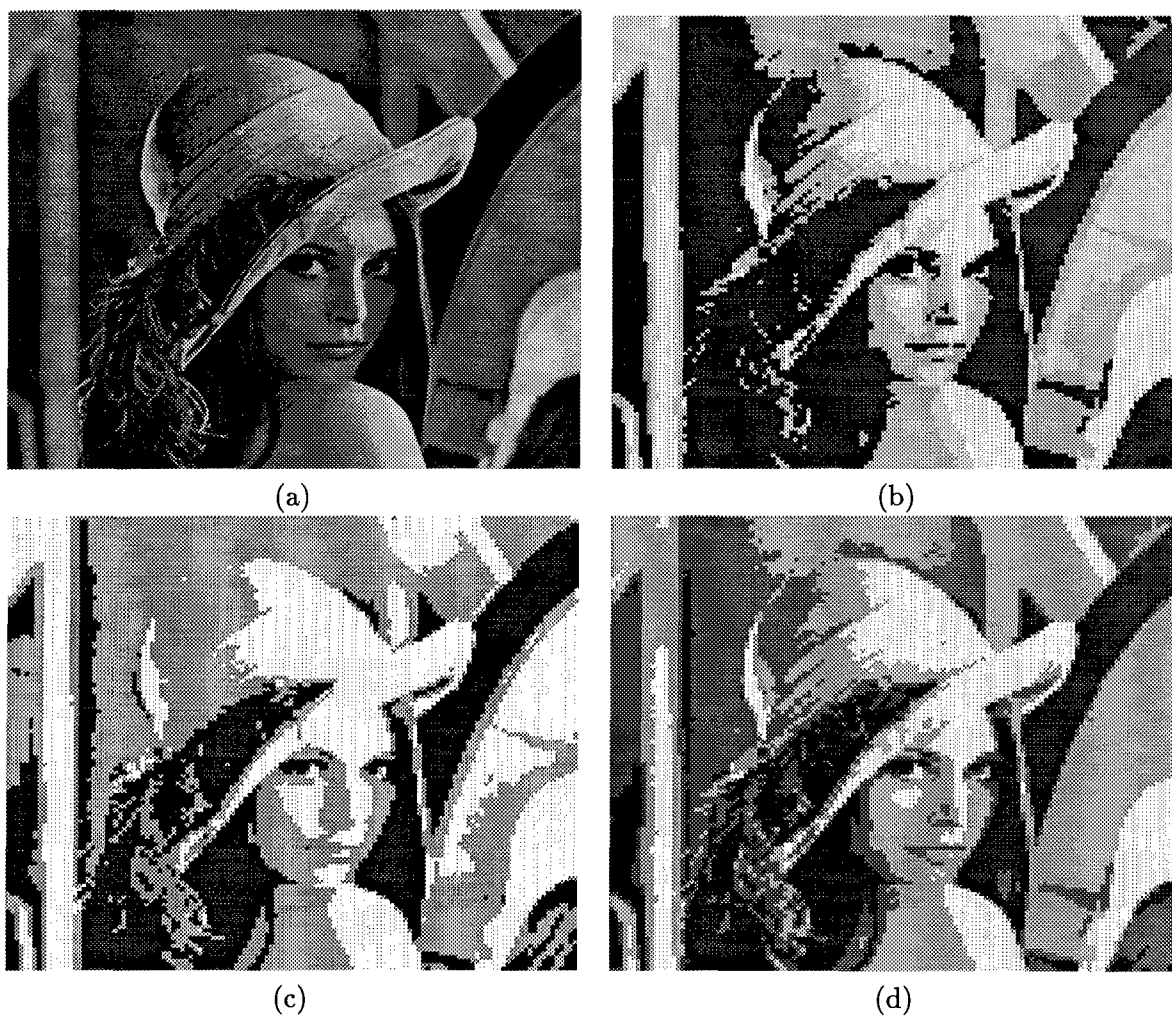
Figure 15. Original and reconstructed Lena images using the different clustering methods. (a) Original Lena image. (b), (c), and (d): Reconstructed image using the four-class codebook generated by WMD, FCM, LBG methods, respectively
