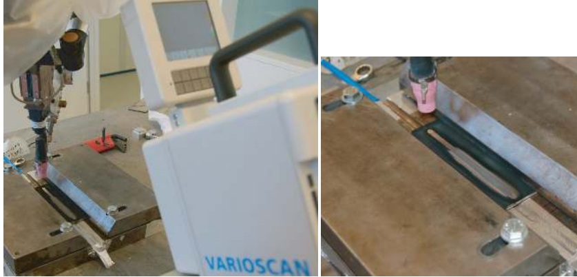
Figure 17: Experimental setup for measuring the surface temperature during a GTA welding process.
