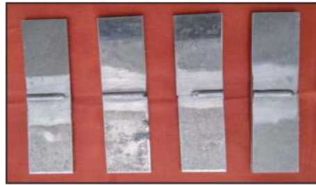
FIGURE 1: TIG-welded AA8006 plates.
