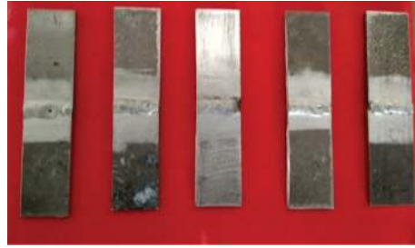
FIGURE 5: Rockwell hardness testing specimen.
