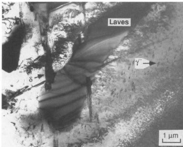
Figure 3 - Bright field TEM micrograph of the DTA sample microstructure. Laves, \delta , and \gamma' are indicated by arrows.
