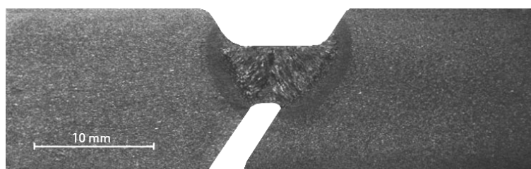
Fig. 5. Cross-section of the P2 test joint with the visible crack initiated in weld root
