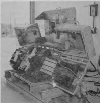
FIGURE 7 - HEAT TREATMENT OVEN USED FOR CRAWLER SHOE REPAIR WELDING
