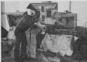
FIGURE 8 - REPAIR WELDING A CRAWLER SHOE
