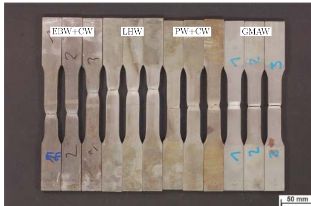
Fig. 3 Overview of all tested flat bar tensile test specimens. The fracture location is always clearly visible
