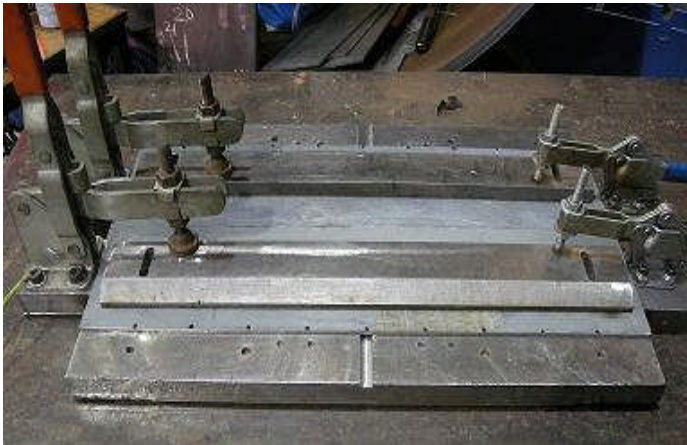
Fig. 2 Clamping arrangement for plates.
