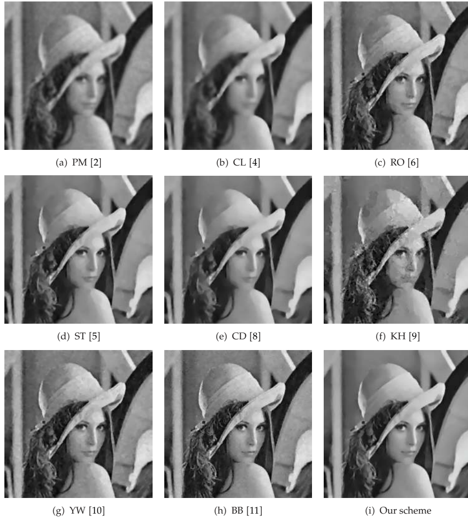
Figure 4: Results of (a) Perona and Malik scheme [2], (b) Catté et al. scheme [4], (c) Rudin et al. scheme [6], (d) Strong scheme [5], (e) Ceccarelli et al. scheme [8], (f) Kusnezow et al. scheme [9], (g) Yu et al. scheme [10], (h) Barbu et al. scheme [11], (i) Our \alpha -ADS scheme.
