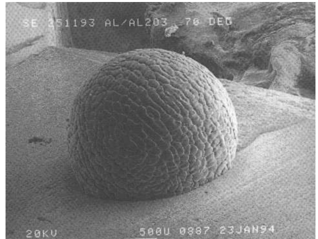
FIG. 1. SEM image of an Al drop on an \text{Al}_2\text{O}_3 surface.
