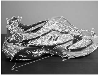
Fig. 2. SIFT keypoints extracted from a 640 \times 480 image of a sneaker. The algorithm found 1533 features shown as white arrows, with size and direction corresponding to feature scale and orientation, respectively.
