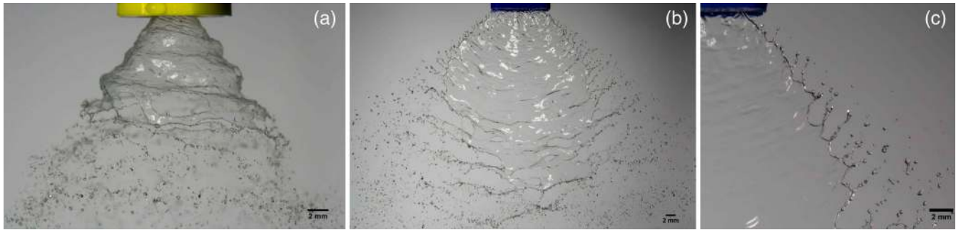
FIG. 1. (a) Picture of the conical nozzle with an operating pressure of 2.0 bar. The Squire wave is clearly visible, with a wavelength in agreement with the prediction. (b) The flat fan nozzle at 2.0 bar, with flapping and breakup occurring near the bottom of the picture. (c) Zoomed-in picture of the flat fan nozzle at low pressure (1.0 bar), showing droplets coming from the sheet's rim that are of the order of the nozzle size.
