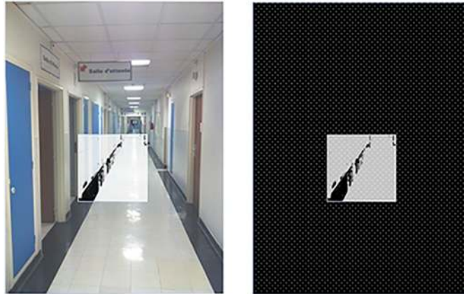
Fig 3. Square representation of the vision field accessed through the prosthesis. On the left you can see that it's only a portion of the whole image, and on the right you can see how the "square image" might be perceived through the device (prior to being converted into electrical pulses that would result in phosphenes) (HK).
