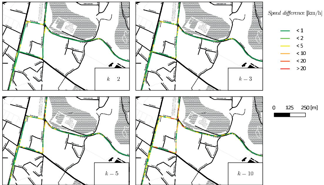
Figure 7. Speed difference for a discretization of factor k mapped to the FCD recorded at 1 Hz. The green color indicates a low speed difference ( < 1 km/h), the red color a high speed difference ( > 20 km/h). A slightly lower sampling rate ( k = 5 ) already results in a severe loss of information; green and red phases alternate frequently. Especially near to road intersections where the car is decelerating or accelerating speed differs by up to 20 km/h from the reference.
