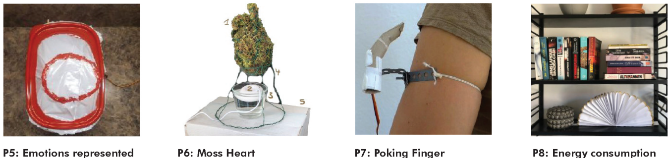
Figure 7: The interactive physicalisations created by P5, P6, P7, and P8. Left: P5 tried to create a mouth which represents the user's emotional state. Middle left: P6 created a moss heart which represents your emotional state. In an app, the user indicates how they feel that day. If they feel good, the moss heart receives water via a humidifier, but if they feel unhappy, it remains dry. The physicalisation thus is a literal representation of how your heart 'feels', with positive feelings resulting in a green and lively moss heart and negative feelings in a brown heart. Middle right: P7's Poking Finger: "a satirical data-object, aims to make people aware of the omnipresent social control technologies". This is a wearable to be worn on the upper arm and connected to the phone. It will tap the user three times to indicate calendar notifications for activities and appointments, continually tap until an incoming call is answered, and poke when the calendar indicates a new work task. One could also connect to somebody else's calendar, thereby experiencing other people's daily rhythm of busyness. Right: P8's physicalisation shows your energy consumption. When fully folded out, it emits light (like a lamp), indicating your energy consumption is low. As the user consumes energy, the device slowly folds and the light dims, until fully closed and dimmed.
