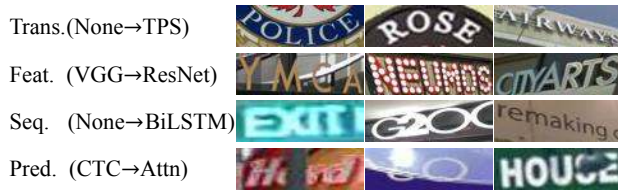
Figure 7: Challenging examples for the STR combinations without a specific module. All STR combinations without the notated modules failed to recognize text in the examples, but upgrading the module solved the problem.
