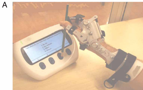
Figure 1 Disease monitoring and messaging device setup with telephone in patient's home. (A) Device adapted for individual with hand impairment.
