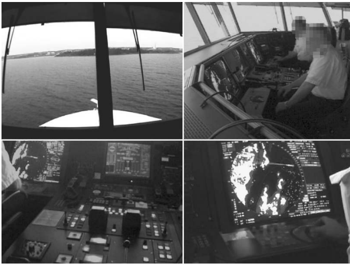
Figure 22: The four video cameras used on the high-speed ferry. Upper left: forward view. Upper right: captain and first mate. Lower left: instrumentation. Lower right: monitor with electronic charts and RADAR.
