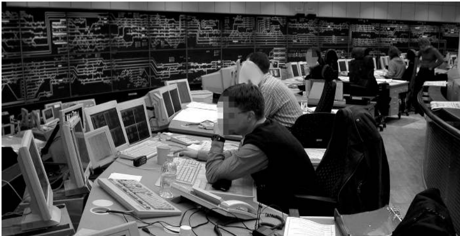
Figure 4: Train dispatchers busy controlling the traffic situation by integrating information and making decisions. Each dispatcher's desk contains at least six monitors, three keyboards and several communications systems. Furthermore, all dispatchers share an entire wall covered with large monitors.
