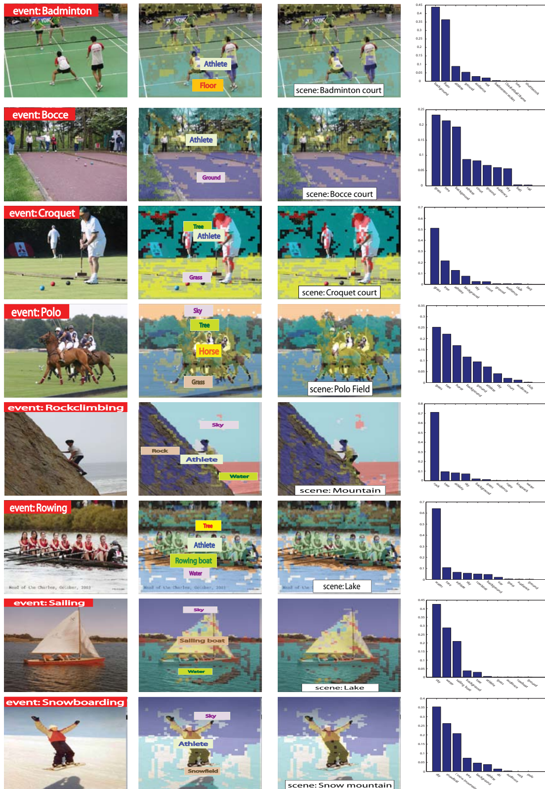
Figure 6. (This figure is best viewed in color and with PDF magnification.) Image interpretation via event, scene, and object recognition. Each row shows results of an event class. Column 1 shows the event class label. Column 2 shows the object classes recognized by the system. Masks with different colors indicate different object classes. The name of each object class appears at the estimated centroid of the object. Column 3 is the scene class label assigned to this image by our system. Finally Column 4 shows the sorted object distribution given the event. Names on the x-axis represents the object class, the order of which varies across the categories. y-axis represents the distribution.
