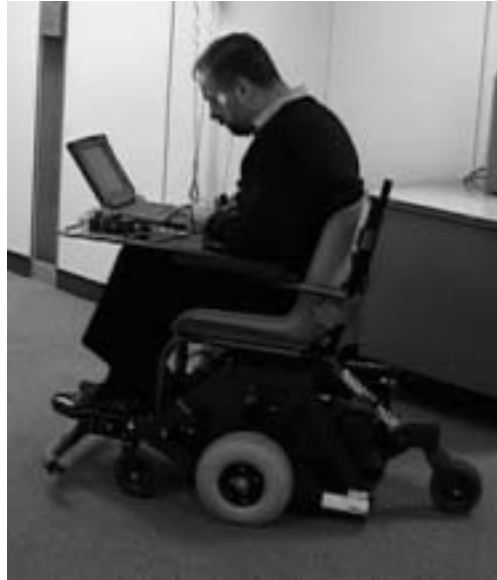
Fig. 5. The robotic wheelchair system being driven using an eye tracking system.
