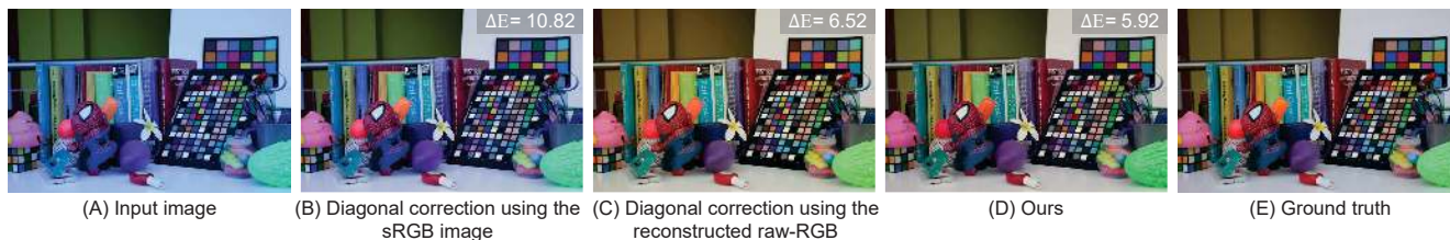
Figure 6. Comparison of our results against applying white balance to the reconstructed raw-RGB image as proposed by [34]. The work in [34] is able to reconstruct the raw-RGB image by embedding radiometric calibration metadata in the sRGB data. By reversing back to the raw-RGB, they can re-apply white balance correctly and then re-render the sRGB image. (A) Input sRGB image. (B) Result of diagonal correction on sRGB color space. (C) Result of diagonal correction on the reconstructed raw-RGB image [34]. (D) Our result. (E) Ground truth image. (A)-(C) and (E) are adapted from [34].
