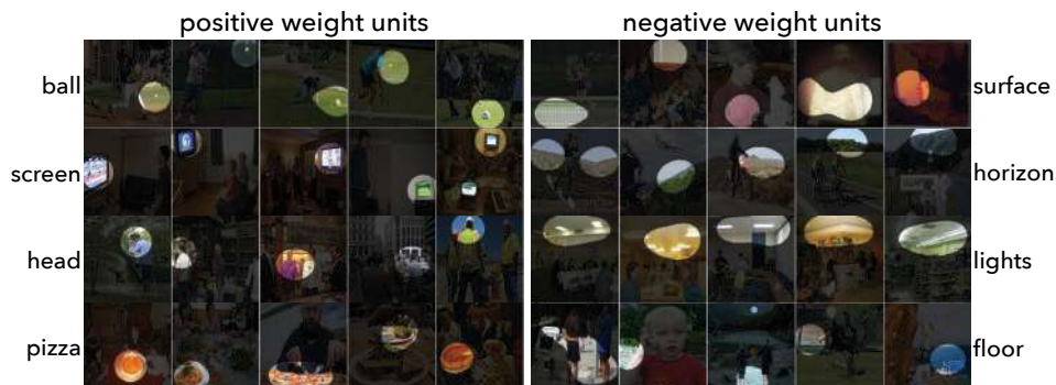
Figure 7: Visualization of saliency units: We visualize several units in our saliency pathway by finding images with high scoring activations, similar to [21]. We sort the units by w , the weights of the sixth convolutional layer (See Section 3.1 for more details). Positive weights tend to correspond to salient everyday objects, while negative weights tend to correspond to background objects.
