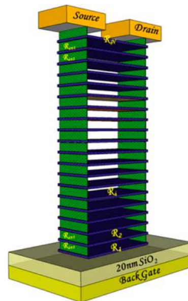
Figure 3. A resistor network based on T-F charge screening and interlayer coupling that describes multilayer two-dimensional systems.
