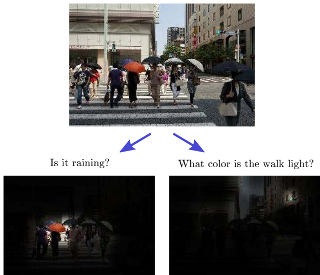
Figure 1. Our goal is to identify the correct answer for a natural language question, such as “What color is the walk light?” or “Is it raining?” We particularly focus on the problem of learning where to look. This is a challenging problem as it requires grounding language with vision and learning to recognize objects, use relations, and determine relevance. For example, whether it is raining may be determined by detecting the presence of puddles, gray skies, or umbrellas in the scene, whereas the color of the walk light requires focused attention on the light alone. The above figure shows example attention regions produced by our proposed model.
