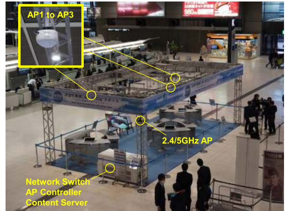
Fig. 10 Experimental Demonstration at Narita International Airport.
