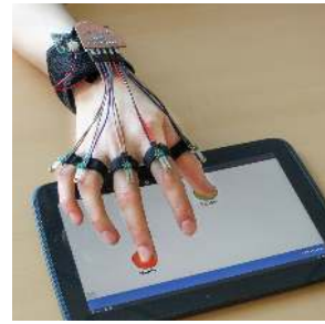
Figure 3: Our wireless device prototype. The micro-controller and battery are attached to the wrist. The sensors are moved to the third phalanx near the palm.
