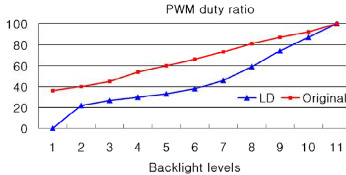
Fig. 10 PWM duty cycle changes for different backlight levels in the ‘Original’ vs. ‘LD’.
