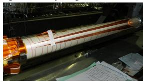
under the US-Japan collaboration developing unique vibration measurement techniques and also novel, compact superconducting spin rotator units, that are basically drop-in replacements for four SuperKEKB ring dipoles.
