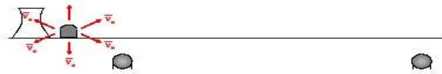
Figure 4: Schematic layout of a two detector reactor neutrino oscillation experiment.
