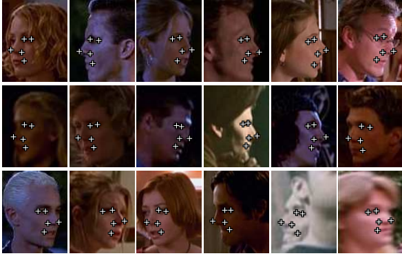
Figure 2. Facial feature localization in profile views. Note the accurate feature localization despite variations in pose between ‘3/4’ view to full profile and challenging lighting.
