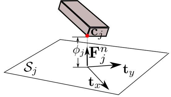
Fig. 3: Illustration of the contact point  $\mathbf{c}_j$ , its distance  $\phi_j$  to the contact surface  $\mathcal{S}_j$ , and the local coordinate frame on the tangential surface, with unit vector  $\mathbf{t}_x, \mathbf{t}_y$ . The complementarity condition holds between contact distance  $\phi_j$  and the normal contact force  $\mathbf{F}_j^n$ .
