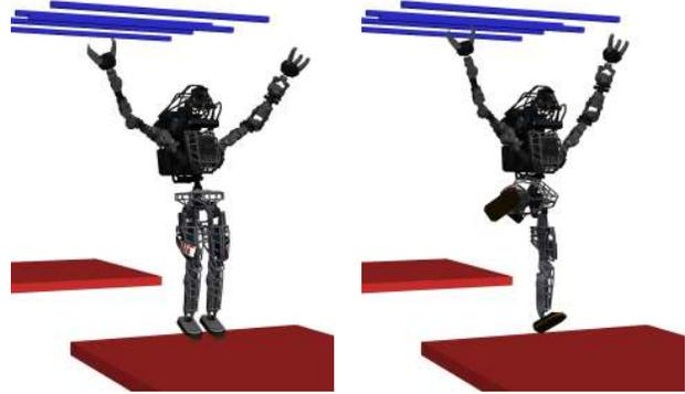
(a) Landing with a fixed mode (b) Landing without a pre-sequence. The left and right toes touch the ground first (left heel touches the ground first)
