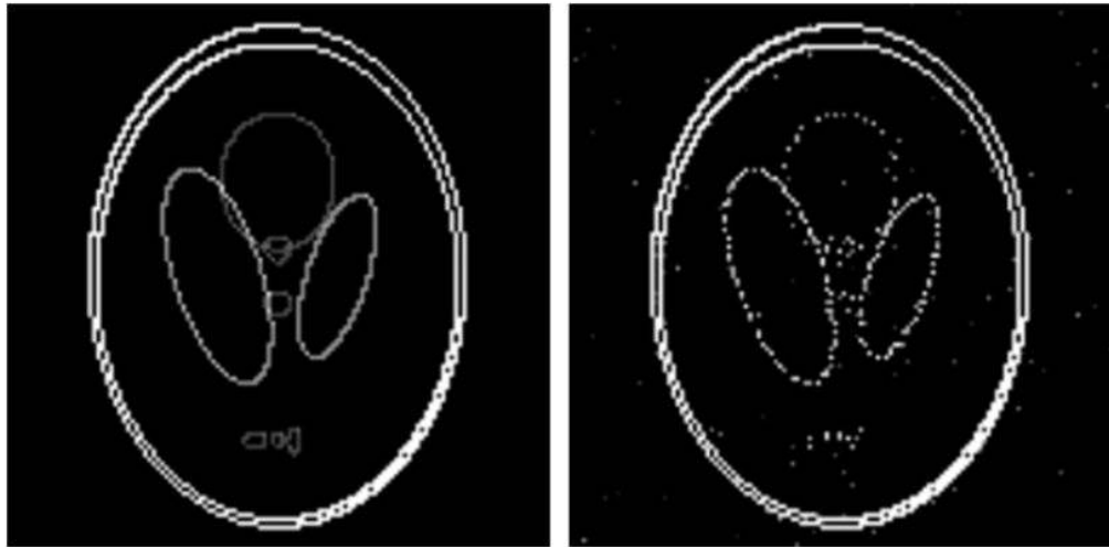
Figure 7. Reconstructed image by IHT-POCS from (left) noiseless data and (right) noisy data with multiplicative Gaussian noise.
