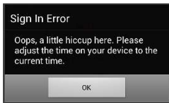
Figure 2: A sample warning message that occurs in an app that is MITM attacked.
